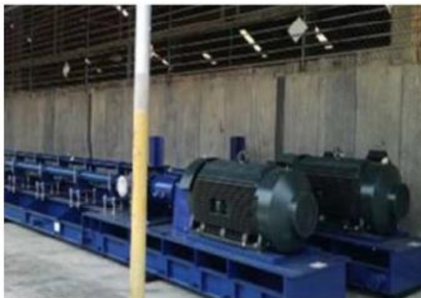
Customer: ECOPETROL COLOMBIA, Llanito Field Project: Water Injection System 2 X VE5500 X 118 STG X 400HP
